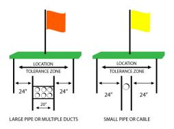
Mechanized equipment is not to be used within the Tolerance Zone until the Excavator has visually identified the precise location of the facility, or has visually confirmed that no facility is present up to the depth of excavation. The Excavator is also responsible to ensure reasonable precautions are taken to avoid any substantial weakening of the facility's structural or lateral support, or both, or penetration or destruction of the facilities or their protective coatings.
