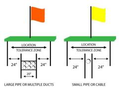
Mechanized equipment is not to be used within the tolerance zone until the excavator has visually identified the precise location of the facility, or has visually confirmed that no facility is present up to the depth of excavation. The excavator is also responsible to ensure reasonable precautions are taken to avoid any substantial weakening of the facility's structural or lateral support, or both, or penetration or destruction of the facilities or their protective coatings.
